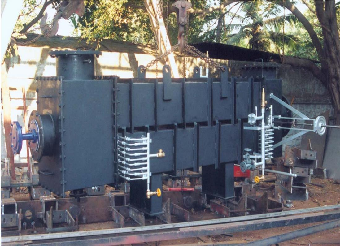
**Figure 1: Matrix Heat Recovery Unit for Steam Generation
